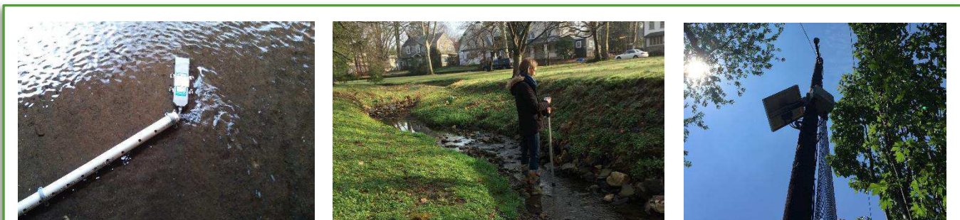
(From Left to Right) Unidata Flow Meter #2, Global Water Instruments Flow Meter, and Vaisala Weather Station
