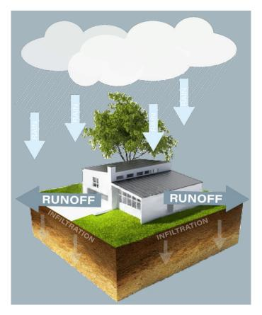
**Figure A** illustrates typical runoff occurring during a rain event in a residential neighborhood. Take note how more runoff occurs than infiltration.
