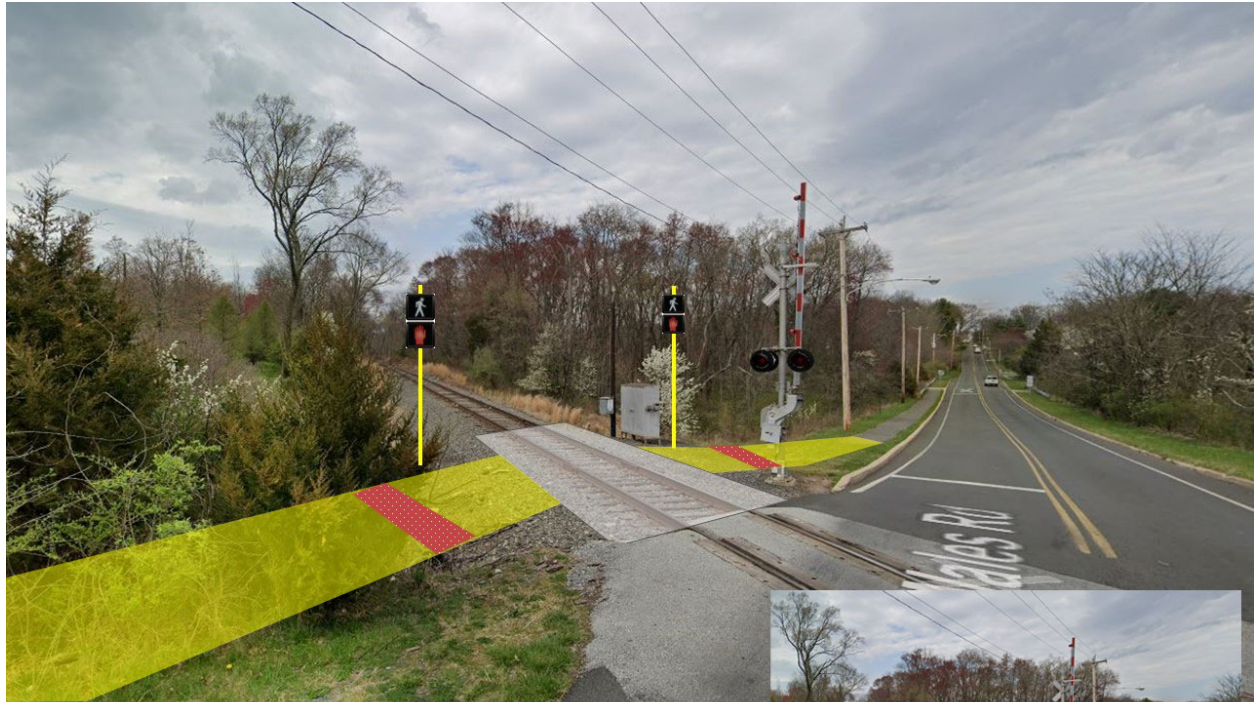
This graphic depicts recommended improvements to two grade crossings of SEPTA's Stony Creek Branch. This is the southernmost of the two crossings, on North Wales Road between Brindle Court and Pulaski Drive. Existing conditions are shown at right
