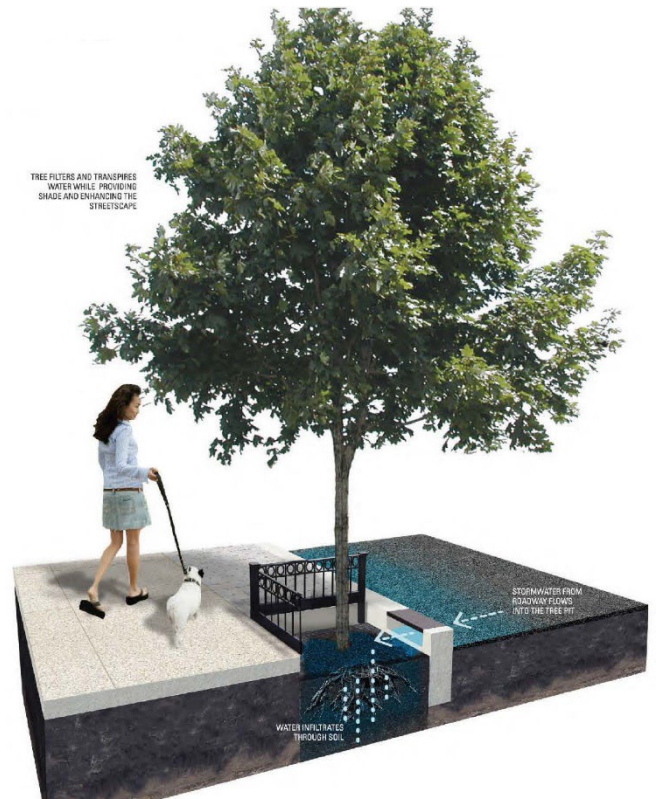
Figure 20. Stormwater tree trench (Philadelphia Water Department)
