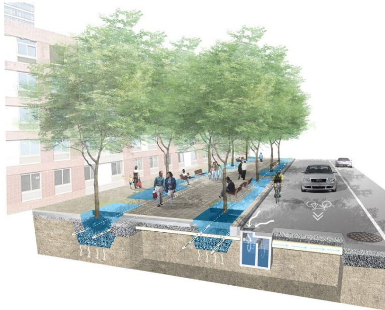
Figure 5. High density green infrastructure integration (Sasaki)
