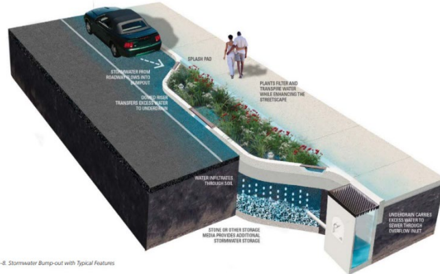
Figure 15. Mid-block Stormwater Bump-out – Philadelphia Water Department
